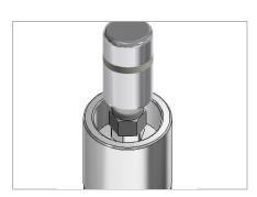
6. Tighten the Dome Nut to secure the data logger in place (fingertight).
