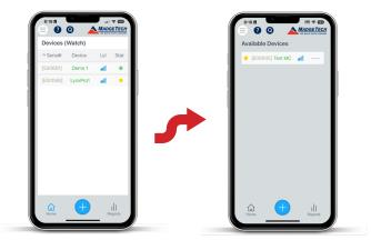
Ensure that Bluetooth is enabled on your smartphone, then press and hold the Bluetooth button on the LynxPro for 3-seconds until the Bluetooth logo appears in the upper left corner. When plugged into external power, Bluetooth will remain on.
