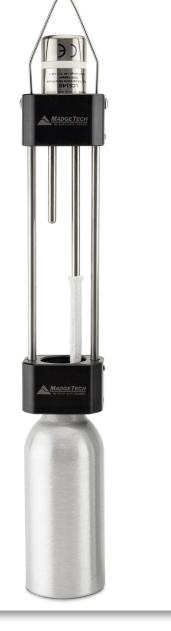
**Note:** Only distilled water is recommended for use in the reservoir bottle.
