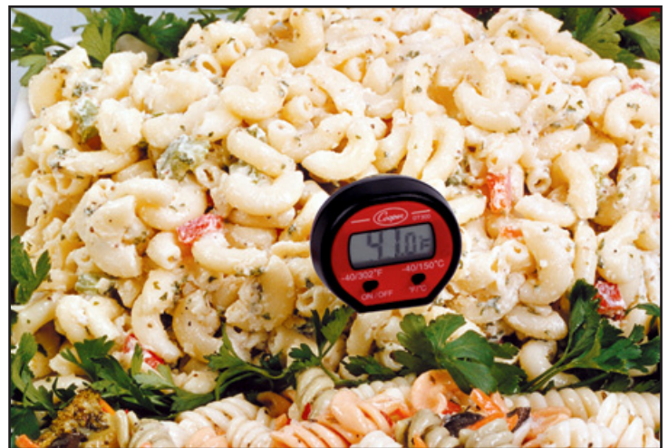
The DT300 digital pocket test thermometer shown checking the internal temperature of a pasta salad dish on a salad bar.
