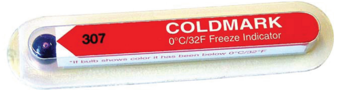
After exposure, bulb turns violet.
